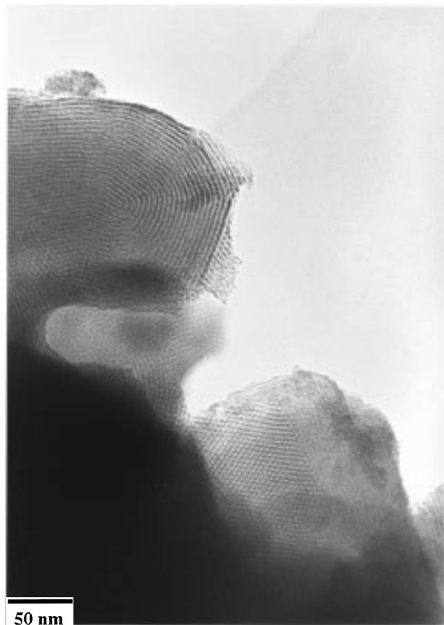
Figure 5. Transmission electron micrograph of zirconium oxide-sulfate showing the hexagonally ordered pores and additionally lamellar structures similar to a fingerprint.
